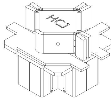
Place, align and fix precisely the cut joint profile as usually to the last installed **Step 3:** joint.
